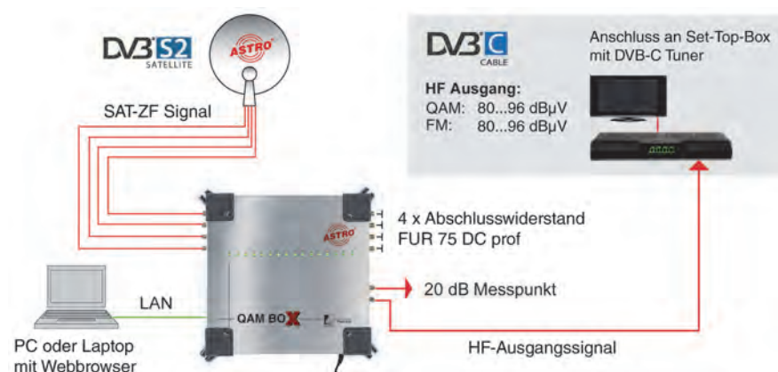
Figure 2: Connecting the QAM BOX
